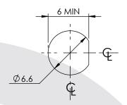
RECOMMENDED TORQUE FOR PANEL NUT: 150 N.cm MAXIMIUM PANEL THICKNESS: 3.2mm
