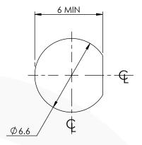
RECOMMENDED TORQUE FOR PANEL NUT: 150 N.cm MAXIMIUM PANEL THICKNESS: 6mm
