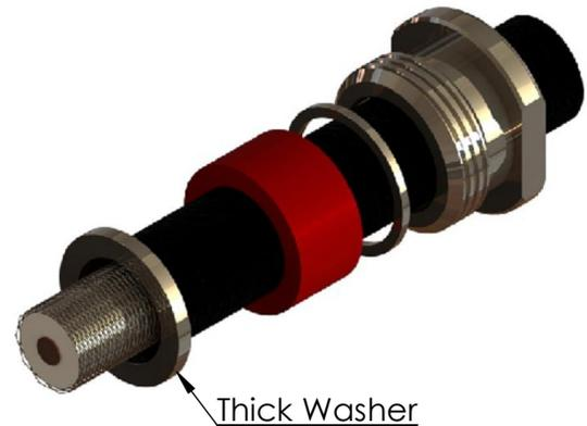
4. With the Braid fanned out evenly, place the smaller diameter end of the Top Hat contact over cable dielectric/foil. Push the Top Hat contact firmly home up to the Thick Washer, thereby clamping the Braid between the Large diameter of the Top Hat and the Thick Washer. When Pushing the Top Hat home you must ensure that the smaller diameter of the Top Hat contact has successfully passed between the cable dielectric/foil and braid of the cable.
