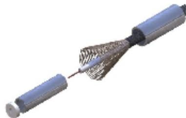
1. Slide centre contact onto cable conductor up to the insulator & sleeve
