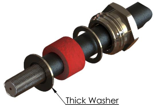
4. With the Braid fanned out, place the tapered diameter of the Top Hat contact over cable dielectric. Push the Top Hat contact firmly home up to the Thick Washer, thereby clamping the Braid between the large diameter of the Top Hat contact and the Thick Washer. When pushing the Top Hat contact home, you must ensure that the smaller diameter of the Top Hat contact has successfully passed between the cable dielectric and braid of the cable.
