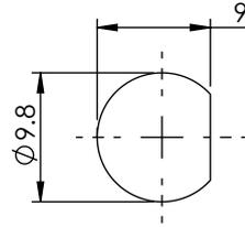
MAX RECOMMENDED PANEL THICKNESS = 4.5mm
